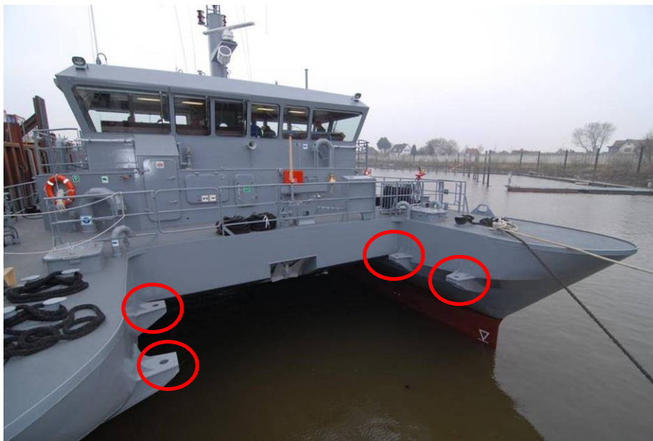
Figure 9: 20' container storage for modules
