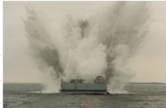
Figure 7: Full load shock trials on test section
