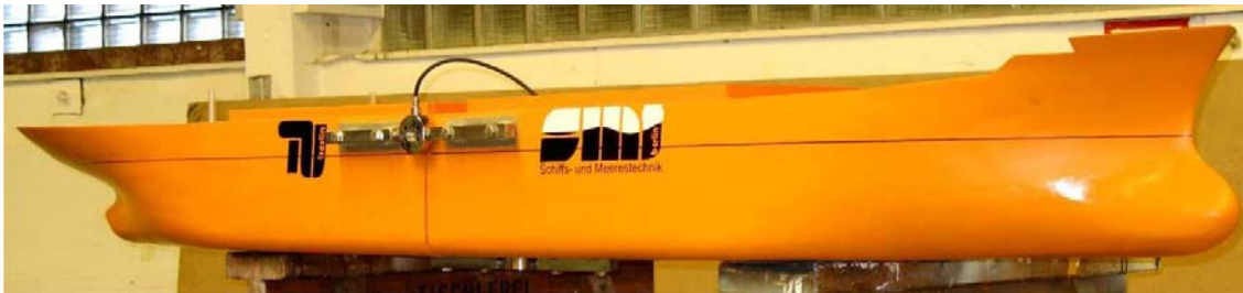
Figure 1: Wooden model of the Bulk Carrier (scale 1:70) subdivided into two segments at the mainframe to measure the vertical wave bending moment.
