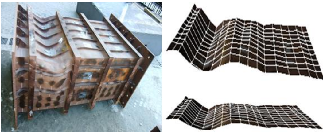
Figure 9: Experimental and photogrammetric decks surfaces after test, first specimen
