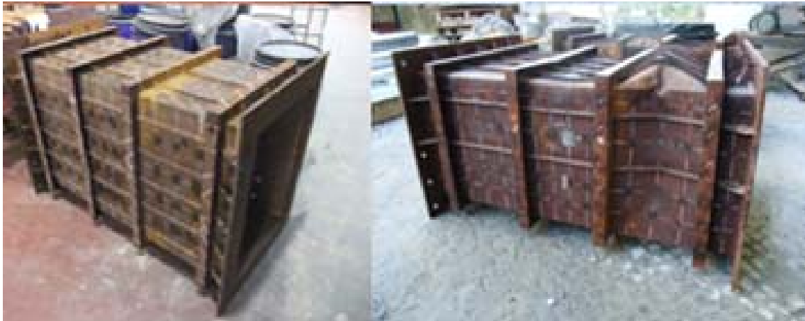
Figure 5: Third box girder, before and after the tests
