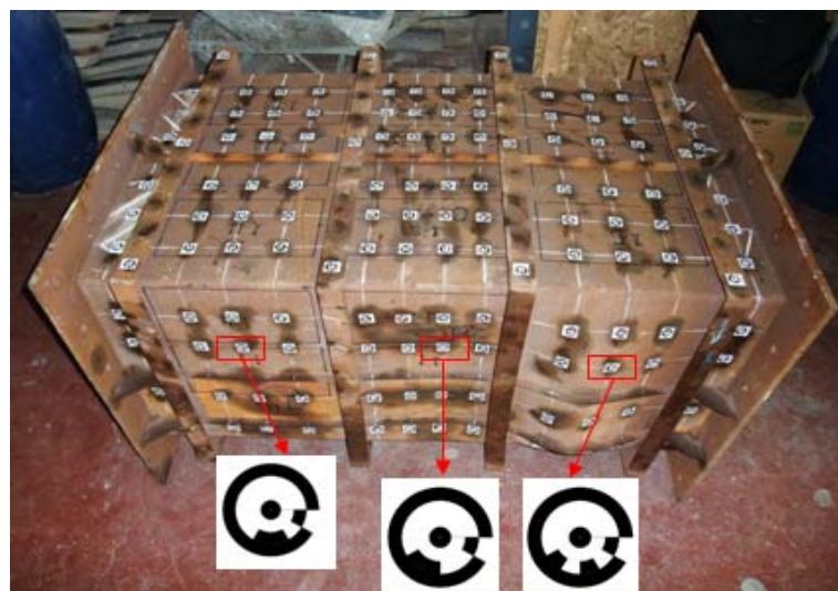
Figure 7: Coded targets attached to the box girder
