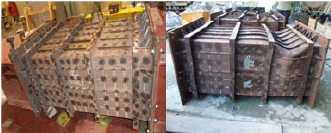
Figure 3: First box girder, before and after the tests
